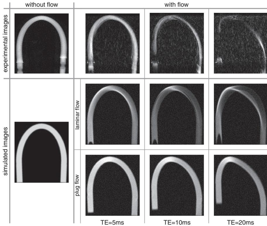
**Fig. 7.** Comparison of experimental and simulated MR images of the U-bend tube geometry. First- and second-row images (experimental and simulated) were acquired with laminar flow with velocity of  $0.38 \text{ ms}^{-1}$ . Moreover, to show difference in displacement effect for various flow patterns, the last row contains simulated images with plug flow with velocity of  $0.76 \text{ ms}^{-1}$ . Frequency encoding in the vertical direction; phase encoding in the horizontal direction.
